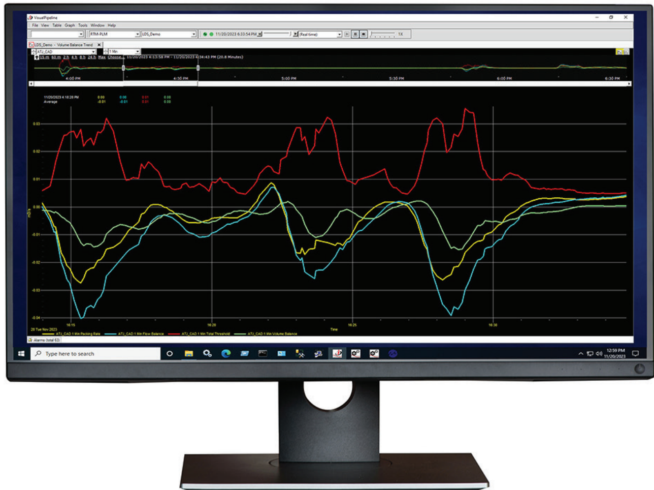
FIG. 4. H 2 operations monitored using real-time modeling software a can capitalize on notification and visualization to identify pipeline leaks more rapidly.
