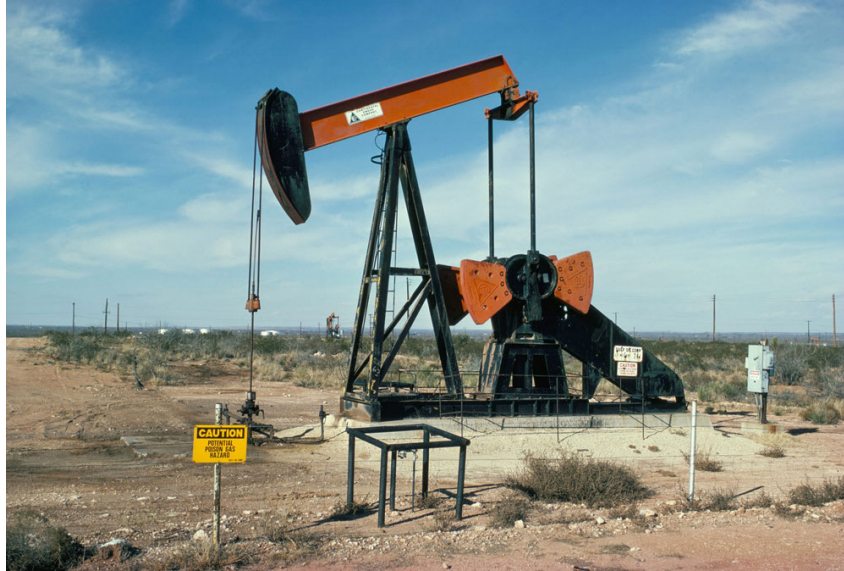
Fig. 5. A rod lift well can experience reduced production due to flumping. Electronic automation and control valves can maintain accurate backpressure on the well, maximizing oil and gas flow.
