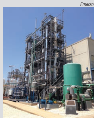
FIGURE 7. The divided wall column at the University of Texas at Austin's Pilot Plant is controlled using WirelessHART networking technology
