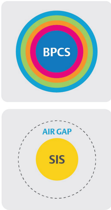
Figure 2: Air-gapped infrastructure separates safety-critical and non-safety-critical SIS but adds extra upkeep to maintain defense-in-depth safety layers on two different systems. Courtesy: Emerson
