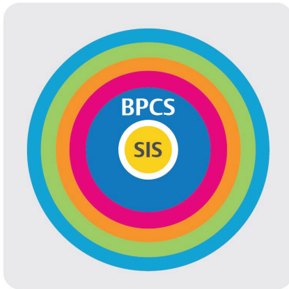
Figure 4: In an integrated SIS architecture, safety-critical functions logically and physically are separated—still complying with ISA and NAMUR standards—yet located on the same system. This eliminates the need to maintain multiple defense-in-depth designs. Courtesy: Emerson
