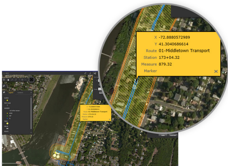
Figure 2. Operators use Emerson's GeoFields™ Facility Explorer to rapidly locate specific pipeline data.
