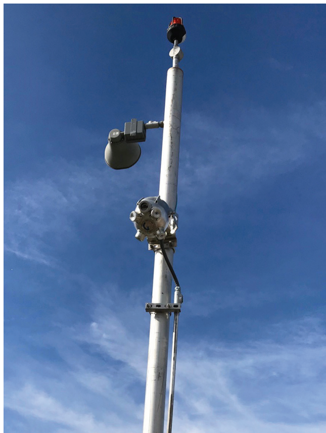
Figure 1. An ultrasonic gas leak detector, such as this one, can capture the sound of a compressed gas leak, and using its directional sensors, help pinpoint the source.
