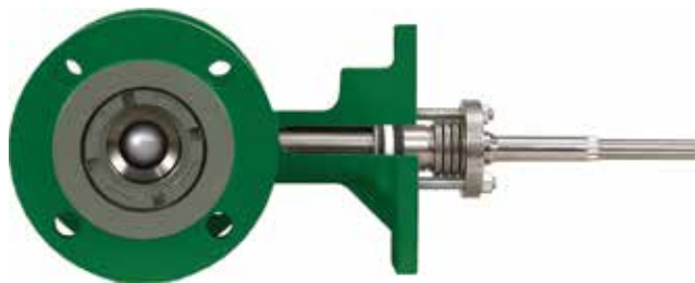
▲ Figure 4. Packing selection is critical for leakfree valve operation. This image depicts the cross section of a live-loaded, low-fugitive-emission packing in an eccentric-plug quarter-turn valve.
