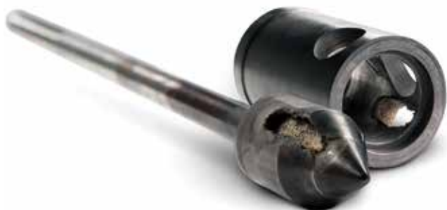
▲ Figure 6. Cavitation and flashing can damage valve components, but may be controlled by using special valve trims.
