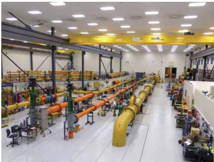
▲ Figure 1. Qualification testing can be done at the valve manufacturer's facility.
