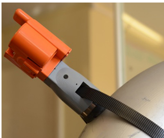
Figure 2. Wall thickness monitoring via UT measurements provides direct metal thickness measurements and detects defects over several decades.
