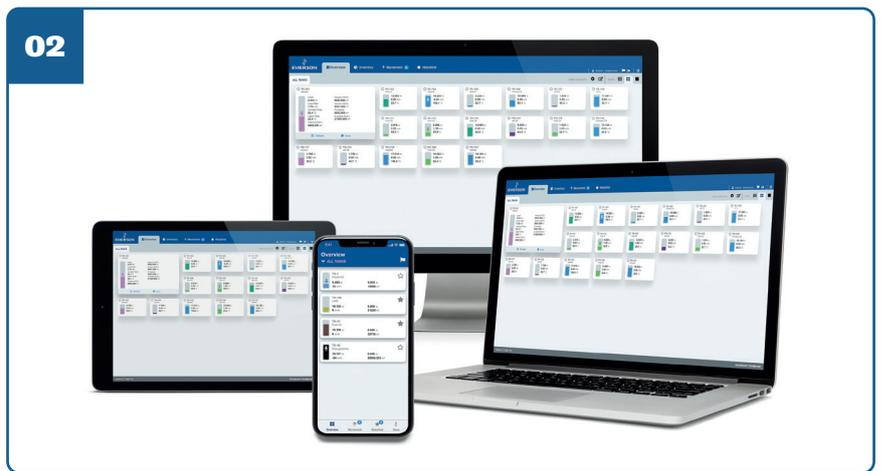
track of tanks more easily. All the tank information is presented on adaptive tank cards, which give an immediate overview of critical inventory data and can differ in size, depending on which tank parameters the user wants to display. Mobile software also enables users to create watchlist groups by clicking an icon on the tank card to quickly and easily bookmark specific tanks of special importance that require close monitoring.
