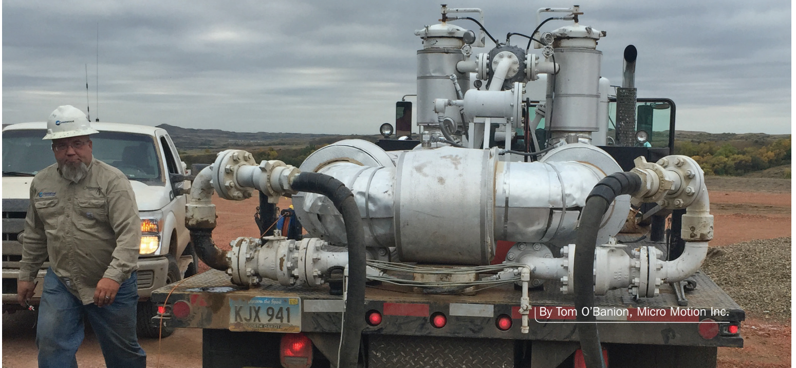
A portable prover on a lease automatic custody transfer unit
