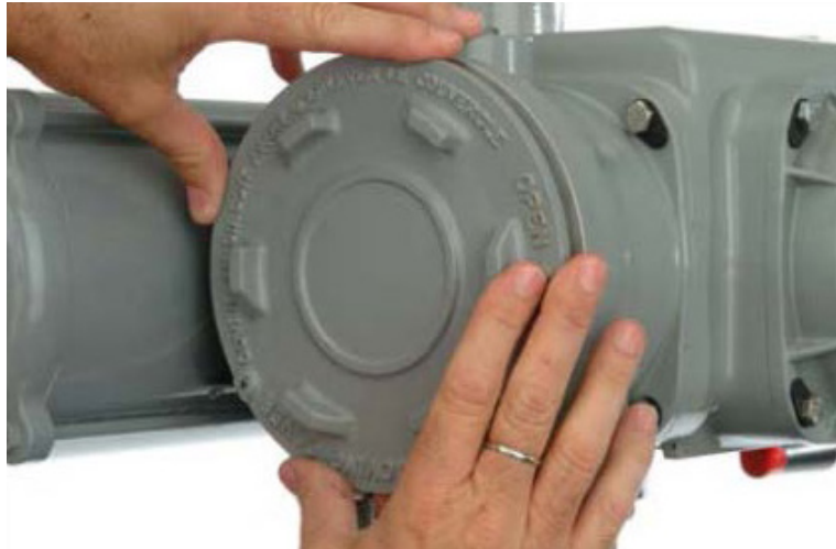
Figure 8 Remove STC Cover Turning Counterclockwise
