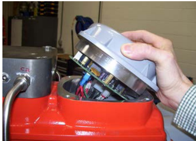
Figure 15 Remove Cover for Limit Switch Chamber
