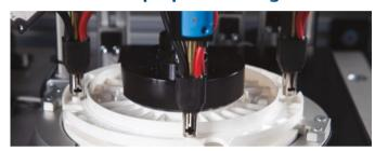
Ability to stake multiple points and polymers simultaneously provide manufacturers with greater design freedom.
