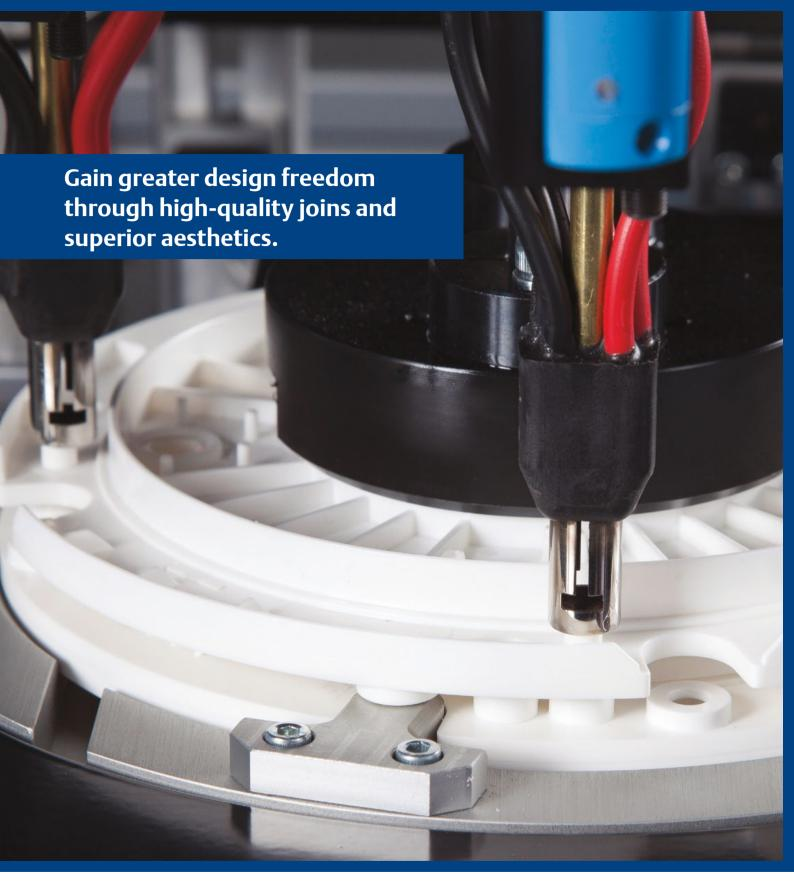
**Branson**<sup>™</sup> **GPX platform**Unique heat staking technology for joining complex, delicate and sensitive plastic components
