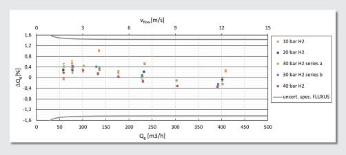
Results of the accuracy tests with pure H2 at the DNV HyLoop facility Groningen
