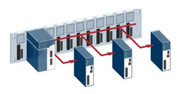
PACMotion is based on PACcore, a multi-core CPU architecture whereby the PAC CPU runs the application program while up to 10 dedicated co-CPUs run the motion algorithms
