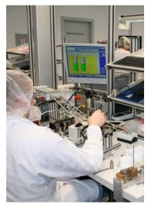
Engineered solutions are manufactured in a Class 8 equivalent clean room environment to minimize contamination, preventing manufacturing rework.
