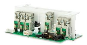
Unique assembly regulates liquid level in the blood chamber of a dialysis machine.
