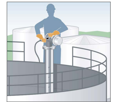
Disconnect existing cabling.
