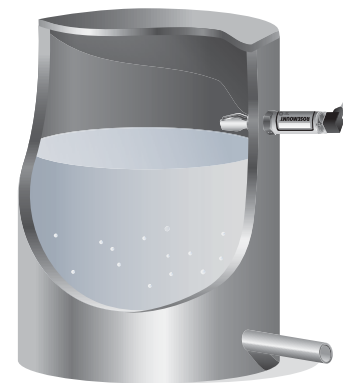
The Vibrating Fork Level Switch is mounted at the high setpoint in each tank.
