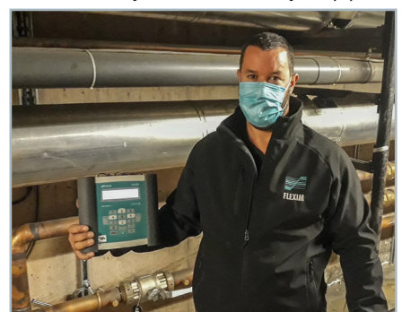
With his portable FLUXUS® G601 CA Energy, Flexim 's service engineer was able to convincingly demonstrate on site the suitability of the non-intrusive ultrasonic technology for the measuring task.
