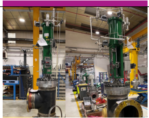
Side and front angles of Fisher FBT 12x20" anti-surge control valve at Cernay, France, manufacturing
