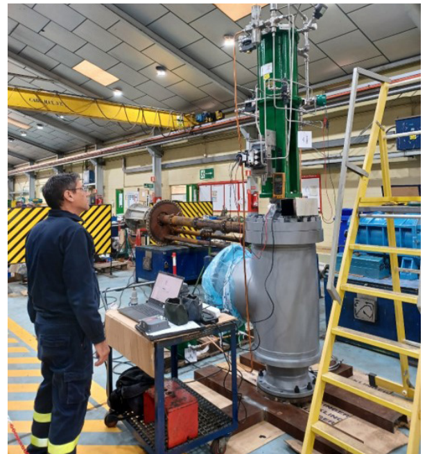
The Fisher Anti-Surge Valve testing at on-site
