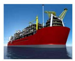
The Prelude FLNG facility will be 488m long, 74m wide and will displace around 600,000 tonnes of water. It will be the largest floating offshore facility in the world.
