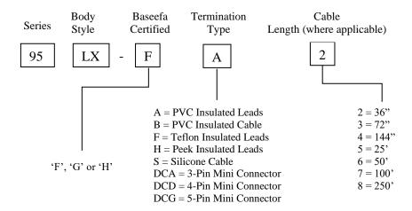
The third character of the Model Number (F, G or H) indicates the temperature classification / maximum surface temperature and ambient temperature range of the equipment, which are as follows:
