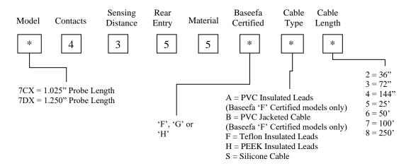
The sixth character of the Model Number (F, G or H) indicates the temperature classification / maximum surface temperature and ambient temperature range of the equipment, which are as follows:
