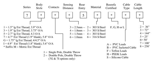
The seventh character of the Model Number (F, G or H) indicates the temperature classification / maximum surface temperature and ambient temperature range of the equipment, which are as follows:
