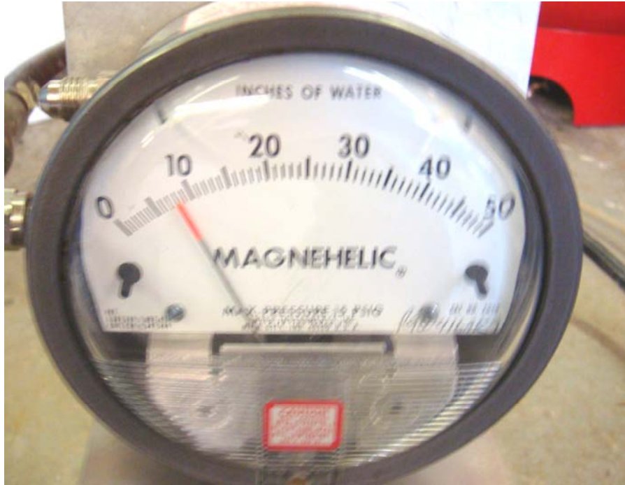
Photograph No. 3 View of Vacuum Gauge during Dust Testing
