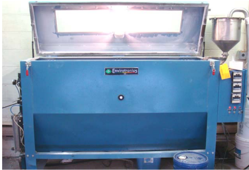
Photograph No. 1 Dust Tightness Test Chamber
