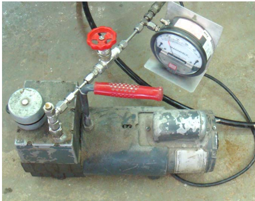
Photograph No. 4 View of Vacuum Pump for Dust Testing
