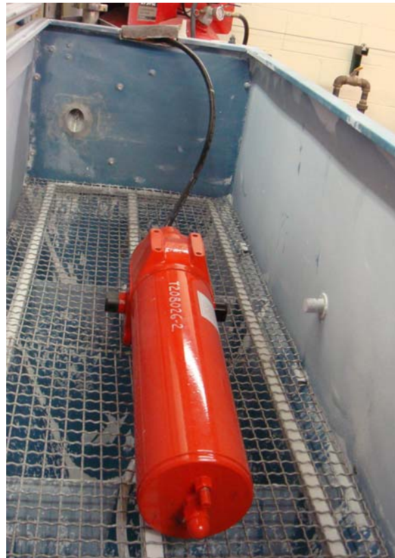
Photograph No. 2 Dust Tightness Test Set-up
