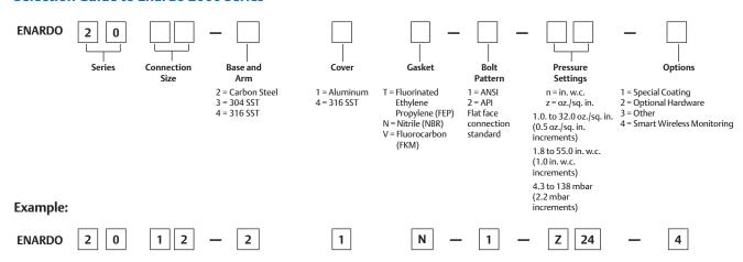
Indicates a 12 in. Emergency Pressure Relief Vent with a Carbon steel base, an aluminum cover with a Nitrile (NBR) gasket, an ANSI 150 lb. Flat Face bolting pattern, with relief pressure of 24 oz./sq.in. and Smart Wireless Monitoring.
