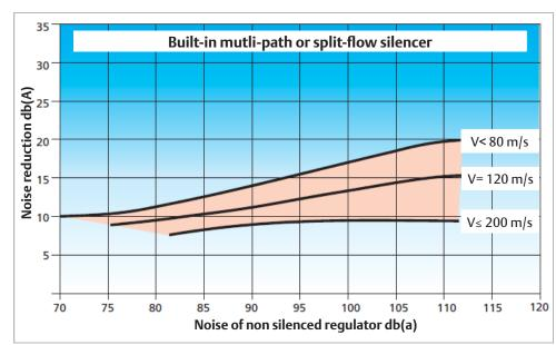
SR - SRS The SRS silencer consists of an SR silencer plus a widened outlet flange in which a second silencer is fitted. The second silencer has an initial multi-path section and a second multi-stage section.
