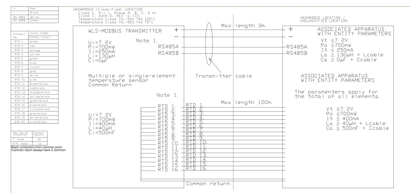
Transmitter and RTD cables are non-detachable. Wires shall be terminated properly at terminal blocks in a suitable junction box according to the installation environment. The junction box shall be mounted directly on top of the WLS tube enclosure.
