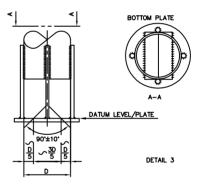
NOTE FOR HIGH ACCURACY MEASUREMENT ( ± 3mm or better) It is important that the installation is done according to iso and api recomendation
