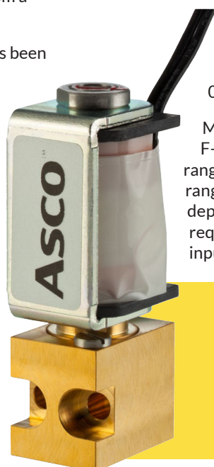
Figure 3. An ASCO 202 Preciflow proportional valve, equipped with an orifice size of just 200 \mu m (0.2 mm), offers the precise actuation required to manage minute changes in airflow and pressure essential to accurate microfluidic delivery. The valve is part of a larger manifold engineered by Emerson. Photo courtesy of Emerson.
