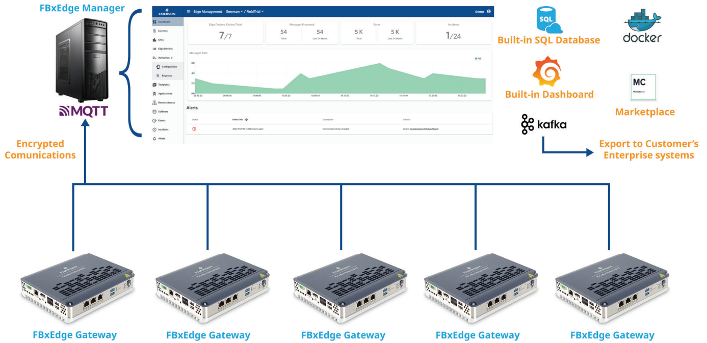
Figure 8: FBxEdge Manager enables FBxEdge users to leverage powerful central management capabilities, including bulk deployment of tags, applications, and remote upgrades.
