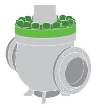
Run your processes for longer with a double offset C-ball valve design that enables non rubbing rotation to eliminate wear and extend maintenance intervals. And if maintenance is required, the <sup>2</sup>XC features a true top entry design with minimal parts for rapid in line maintenance. The entire trim can be removed so repair work can be safely completed outside the pipeline.
