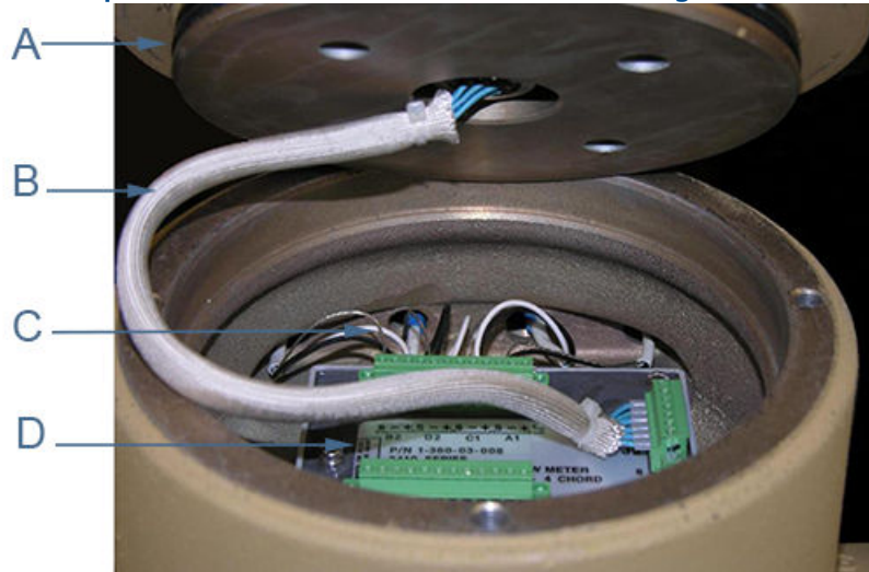
Figure 3-33: Acquisition Module cable and transducer wiring
