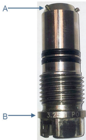
Figure 3-7: Transducer holder length and set screw identification
