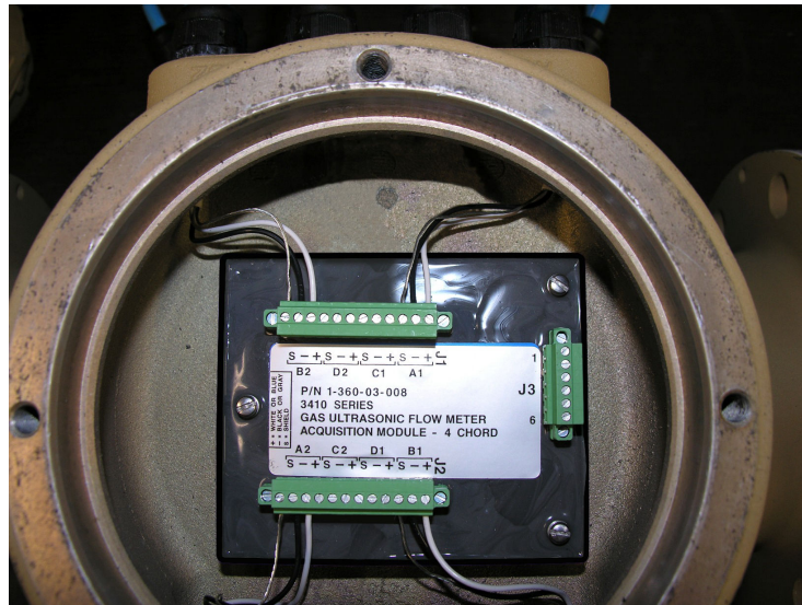
Figure 3-18: Model 3414 Ultrasonic Meter Acquisition Module wiring
