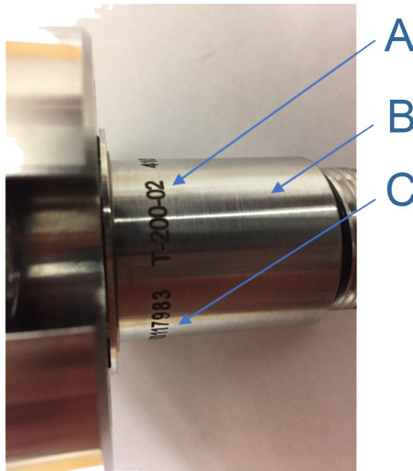
Figure 3-14: T-200 transducer stalk assembly configuration
