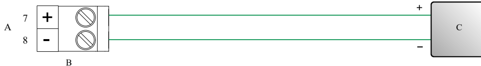
Figure 4-23: mA input wiring (internally powered)
