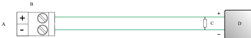
Figure 4-10: Frequency output wiring (internally powered)
