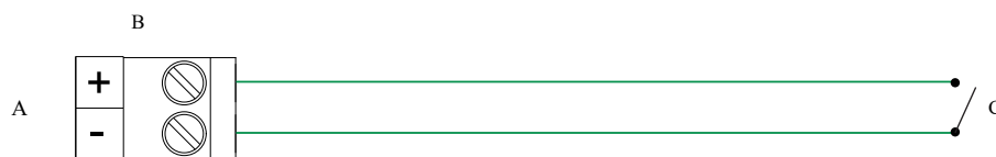
Figure 4-25: Discrete input wiring (internally powered)
