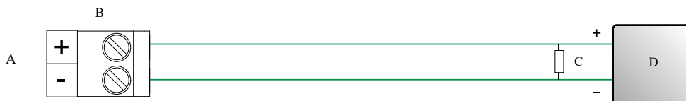
Figure 4-3: mA output wiring (internally powered)
