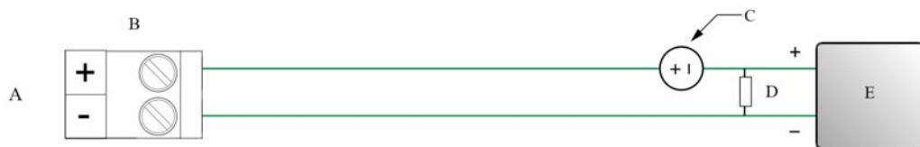
Figure 4-12: Frequency output wiring (externally powered)
