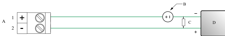
Figure 4-7: mA/HART output wiring (externally powered)
