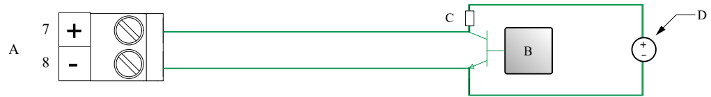
Figure 4-28: Frequency input wiring (externally powered)
