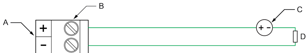
Figure 4-7: DO wiring with a relay or indicator
