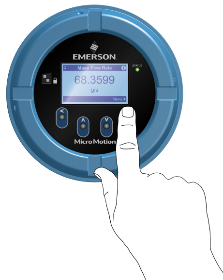
Figure 8-1: Proper finger positioning for activating an optical switch
