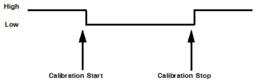
Figure 4-12: Gating configuration parameter State gated, active low
