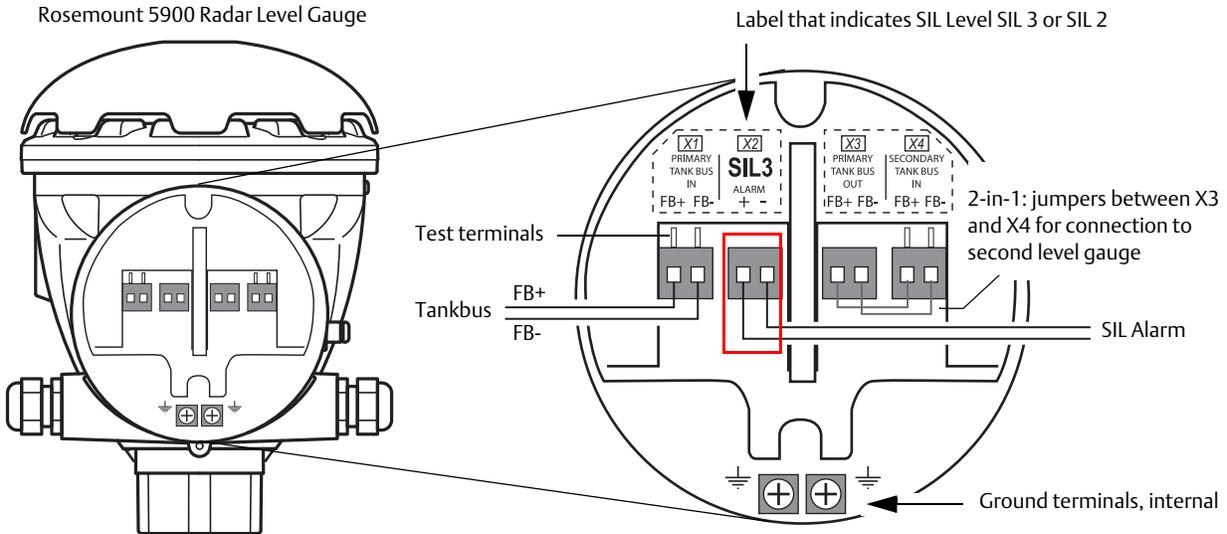
Table 4-2. Rosemount 5900 Terminal Block Connections with SIL Alarm Output
