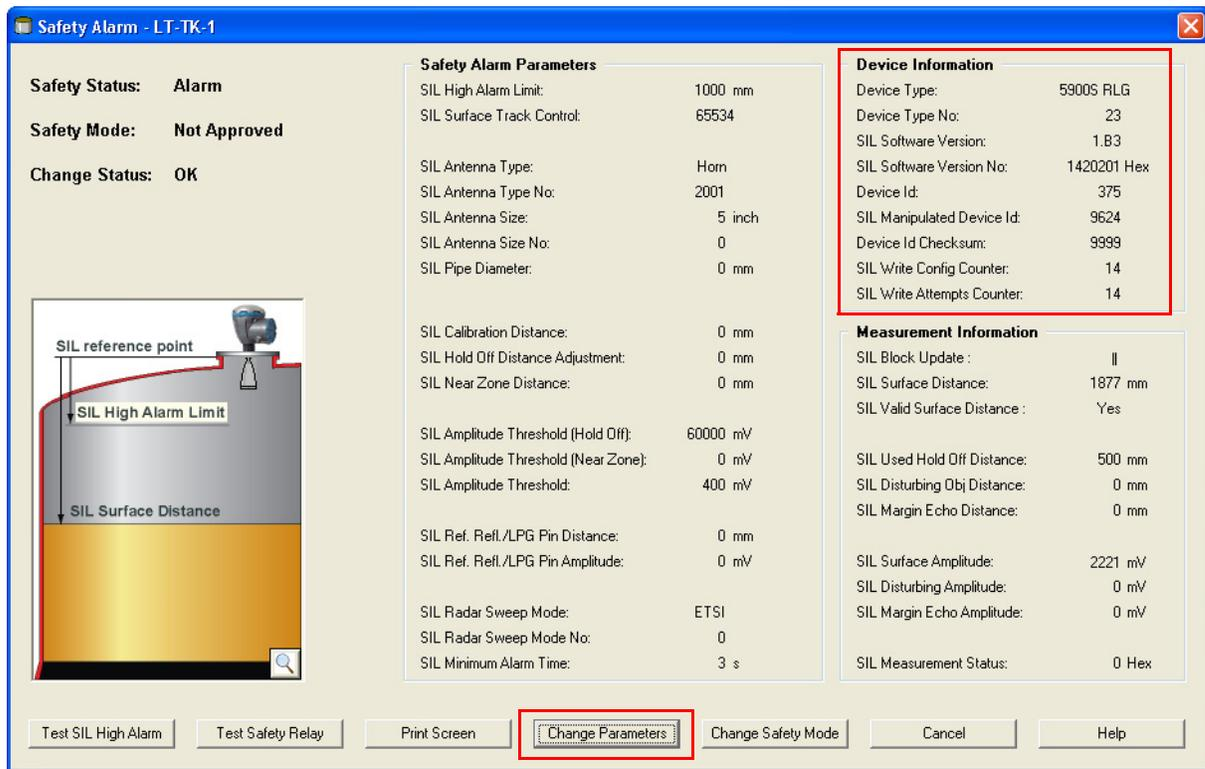
1. In the *Device Information* pane check that the **Device Id** is identical to the Device Id on the main label attached to the Rosemount 5900 housing. For a Rosemount 5900 2-in-1 version, the Device Id is divided in two parts. The first part is for the Primary device and the second for the Secondary device as described in [Appendix C: Safety System Identification](#).
