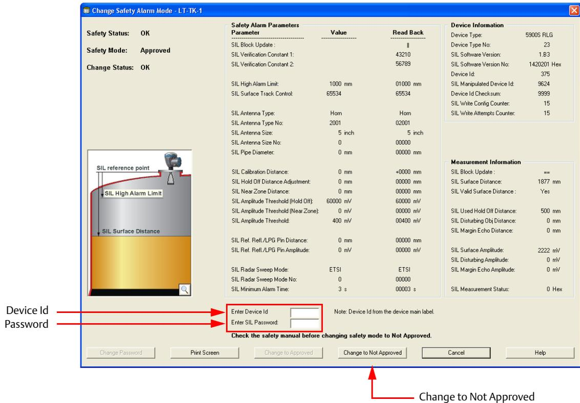
7. In the *Change Safety Alarm Mode* window enter the Device Id and the SIL Password. The default password="1234". The password can be changed once the Safety Mode is set to "Not Approved".
