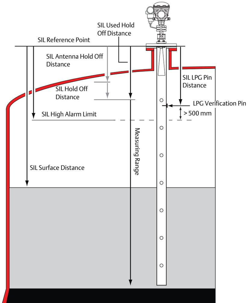
**Figure 4-9. Tank Geometry for a Rosemount 5900 with Parabolic Antenna and Proof Test Reference Reflector**
