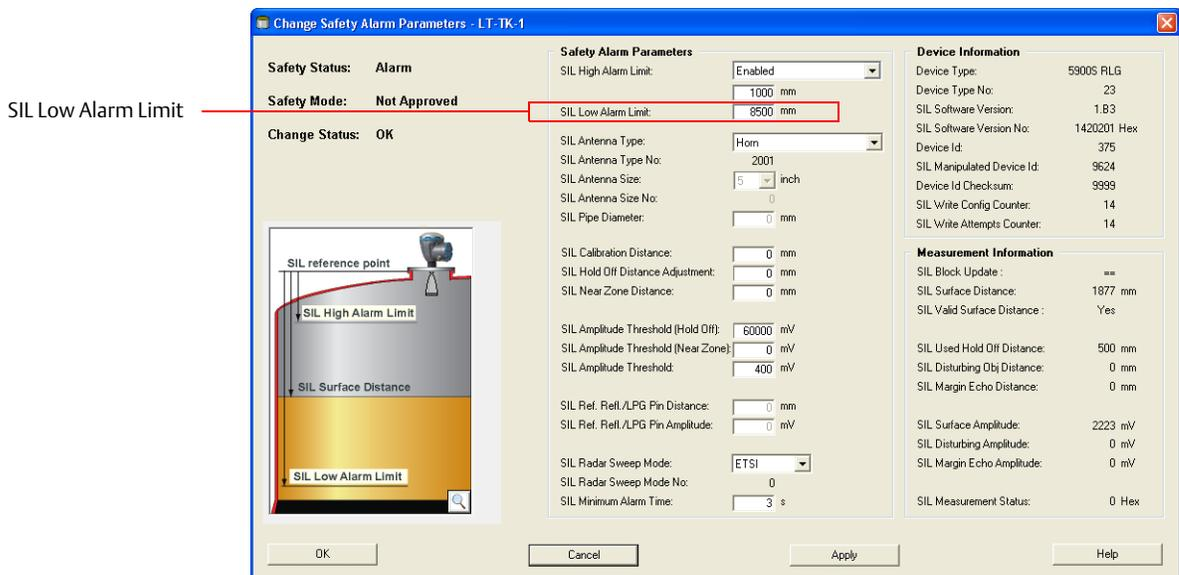
3. Check that the “Surface Track Control” field is changed to **SIL Low Alarm Limit**.
