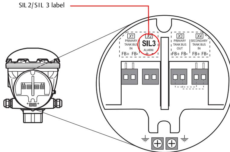
The Rosemount 5900 has different terminal blocks for the SIL 2 and SIL 3 options. The SIL 3 option includes two separate level gauges which need to be configured individually as described in “[Safety alarm setup](#)” on page 19. Check the label in the terminal block to ensure that the Rosemount 5900 has the right option for the required SIL safety level.
