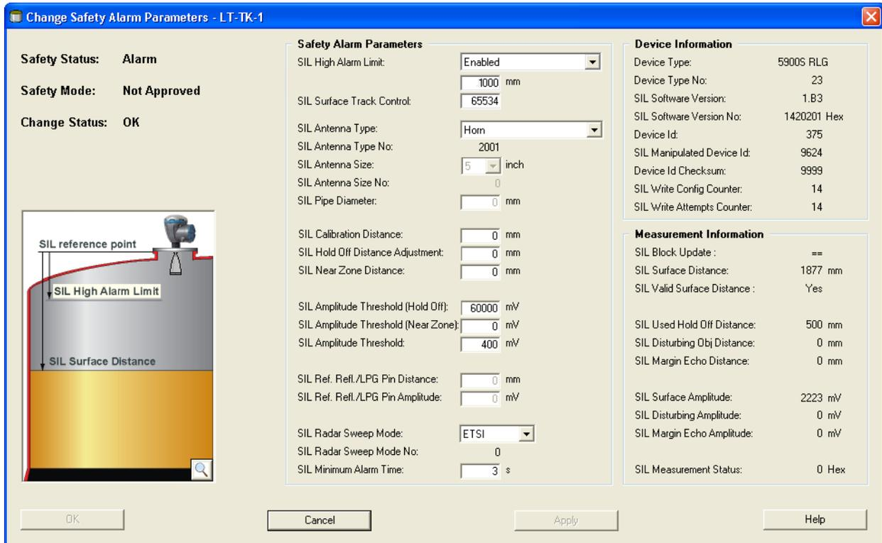
2. In the *Change Safety Alarm Parameters* window, configure the **Safety Alarm Parameters** as described in [Table 4-13 on page 36](#) (see also “Safety alarm parameters and tank geometry” on page 20).
