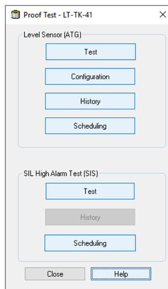
3. In the **SIL High Alarm Test (SIS)** pane, click the **Test** button. The *Safety Alarm* appears.
