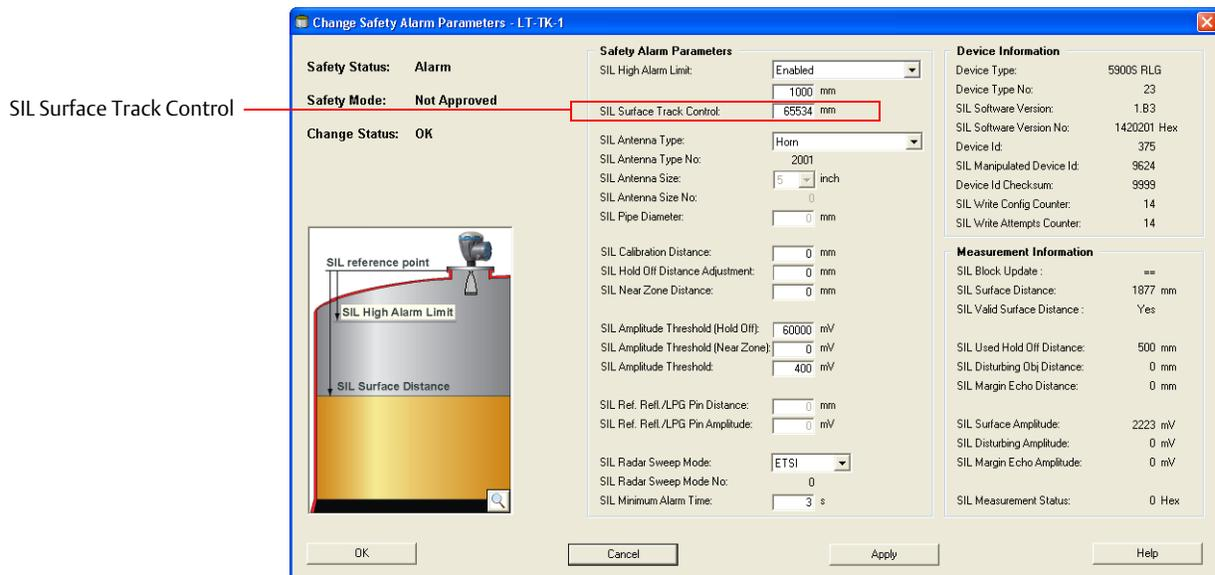
3. Click the **Apply** button to disable SIL Low Alarm Limit and activate SIL Surface Track Control.
