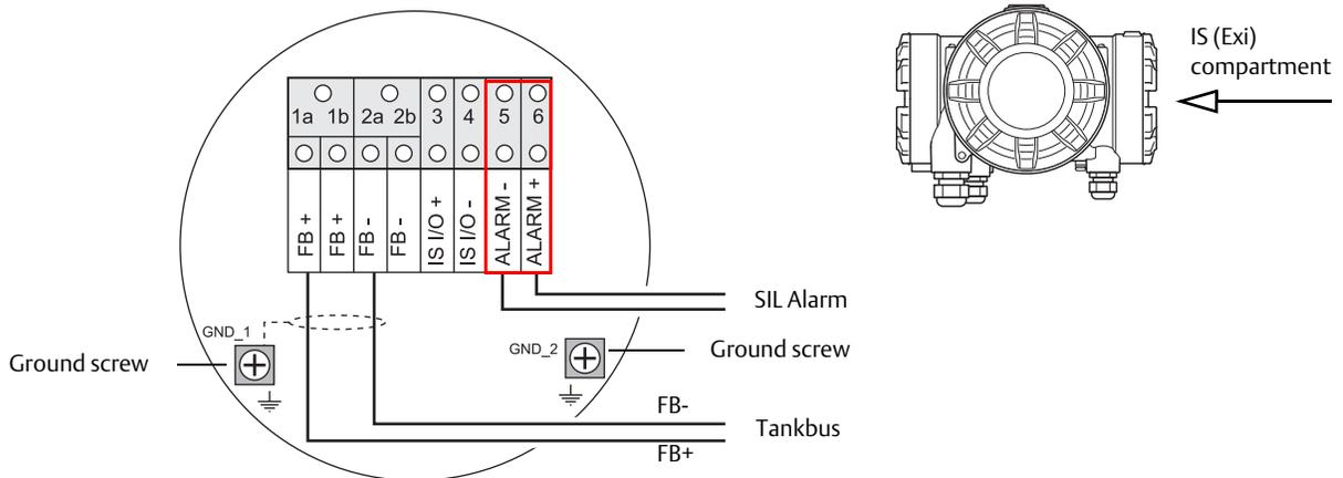
**Table 4-3. Terminal Assignment for Rosemount 2410 IS Terminal Block**
