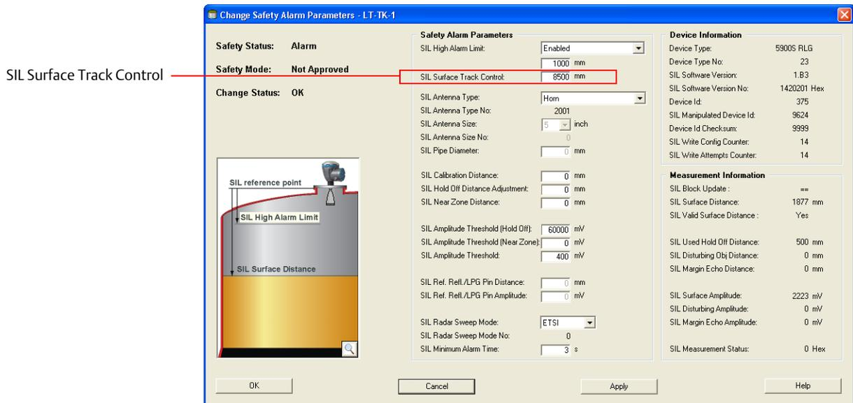
2. In the “Surface Track Control” field, type the desired **SIL Low Alarm Limit** value and click the **Apply** button.
