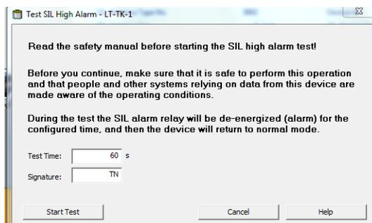
7. In the *Test SIL High Alarm* window, verify the current test time, or change the test time to the desired value.
