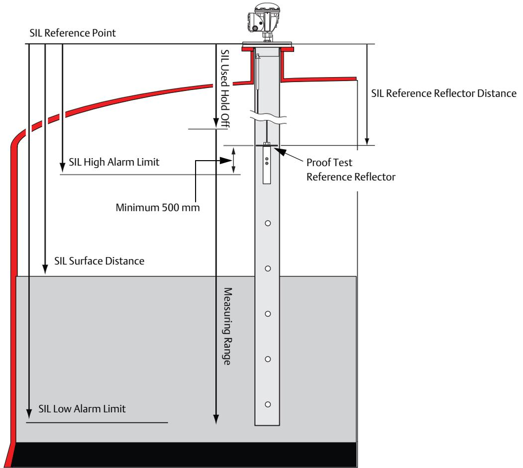
See the Rosemount 5900 Proof Test [Manual Supplement](#) (Document No. 00809-0200-5900) for instructions on how to install and configure a **Proof Test Reference Reflector**.
