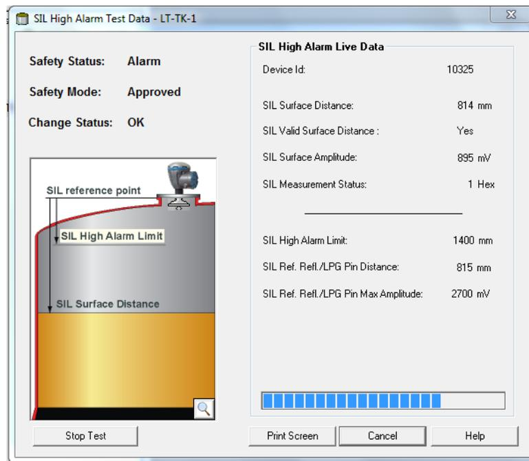
The **Stop Test** button allows you to stop the test before the specified test time has elapsed. You will still be able to fill in the test report form in order to generate a test report file in pdf format. Pressing the **Cancel** button stops the test and no report will be generated. See [Table 5-1 on page 59](#) for information on the various Safety Alarm Parameters displayed in the *SIL High Alarm Test Results* window and in the test report.
