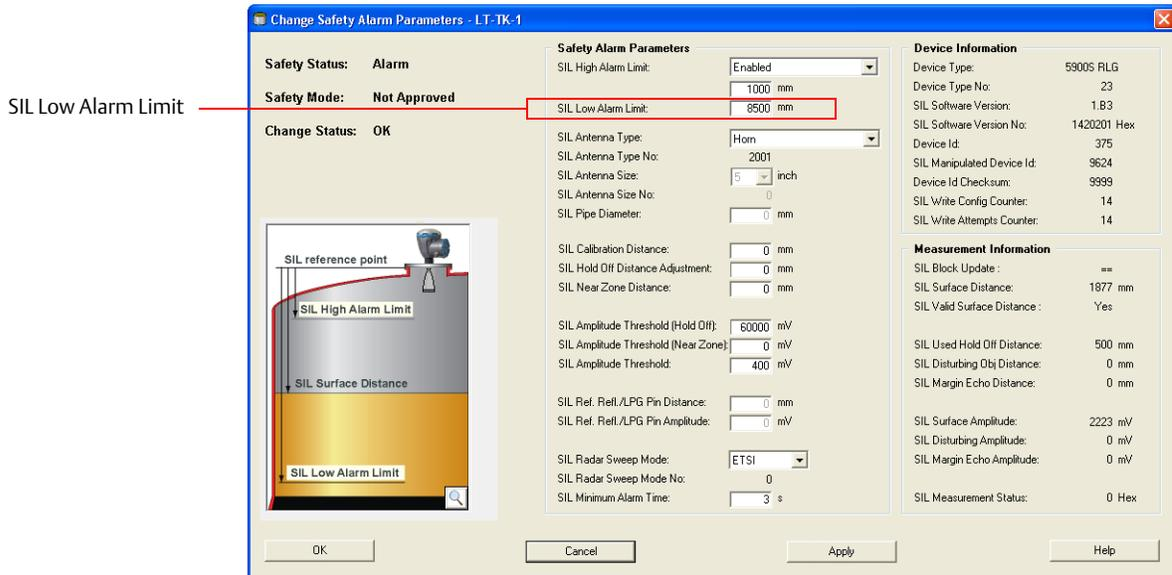
2. In the “SIL Low Alarm Limit” field, type the desired value for **SIL Surface Track Control** (65534 or 655535, see [Table 4-13 on page 36](#)).
