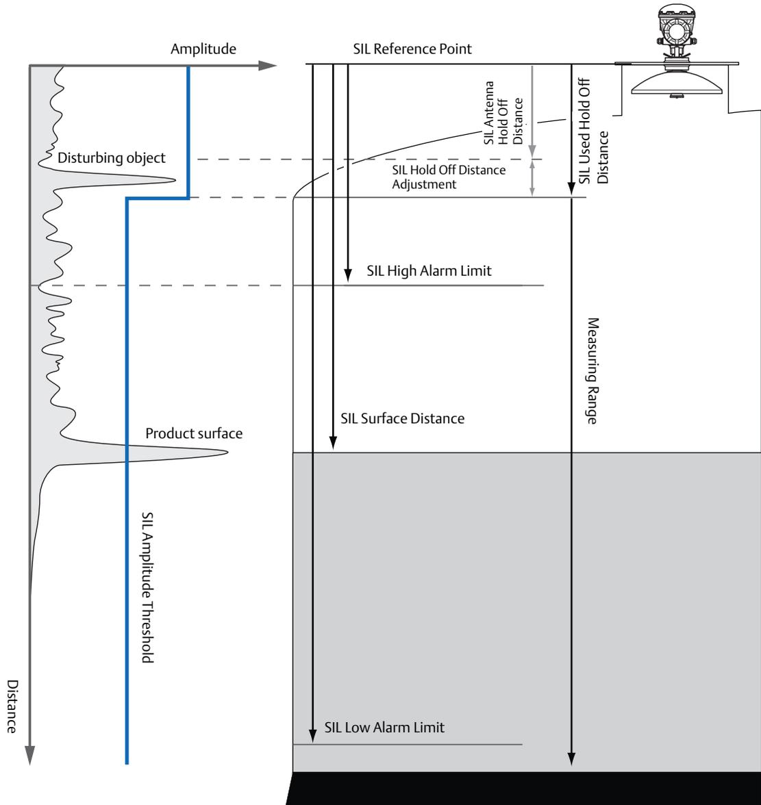
Figure 4-13. Amplitude Threshold in Tank with Rosemount 5900 Radar Level Gauge and Reference Reflector
