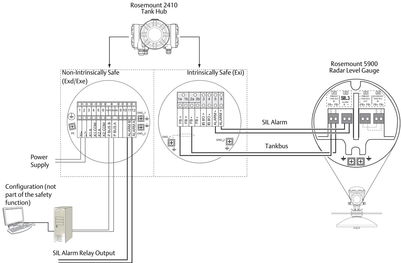
See installation drawings as specified in [Table 4-1 on page 13](#) for more information on wiring the Rosemount 2410 Tank Hub and the Rosemount 5900 Radar Level Gauge.
