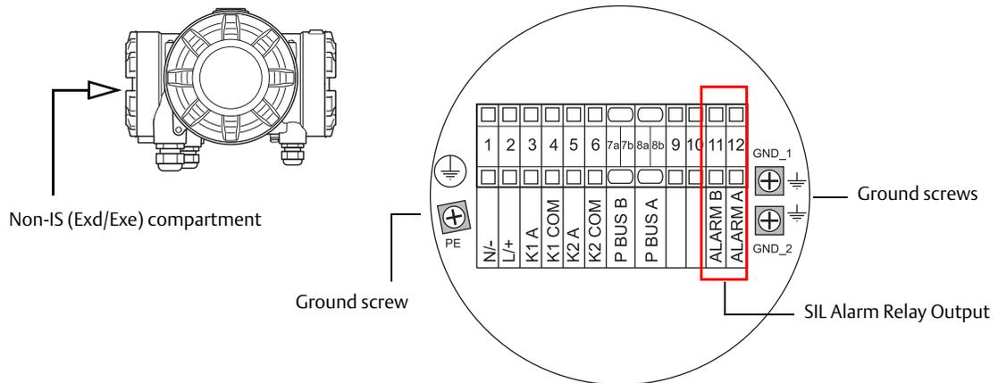
Table 4-4. Terminal Assignment for Rosemount 2410 non-IS Terminal Block
