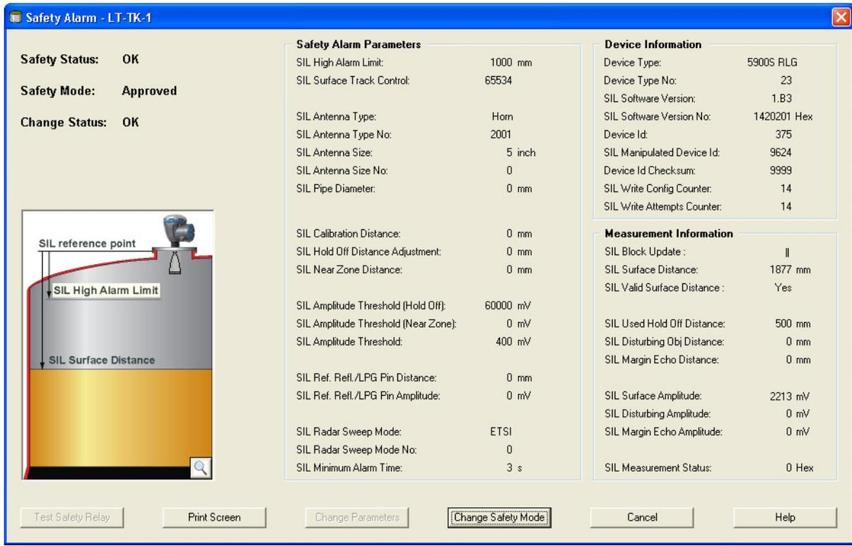
11. Click the **Print Screen** button to print a copy of the current *Safety Alarm* window. The printed copy can be used at a future occasion to check that no changes have been done to the SIL Rosemount Tank Gauging Safety System since last time it was configured.
