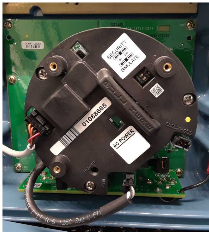
Figure 6-1: Electronics stack and hardware switches
