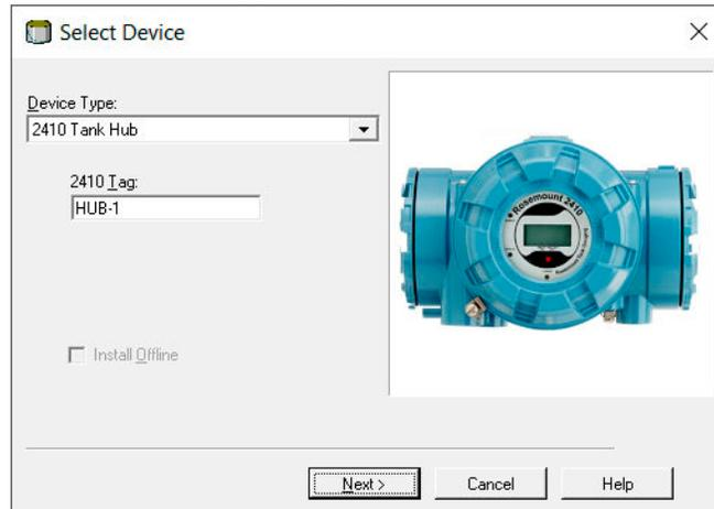
4. Type a name in the 2410 HUB Tag input field. The tag will be used as an identifier for the Rosemount 2410 Tank Hub in various windows and dialogs.
