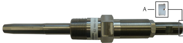
Figure 7-6: Remove cable protection
