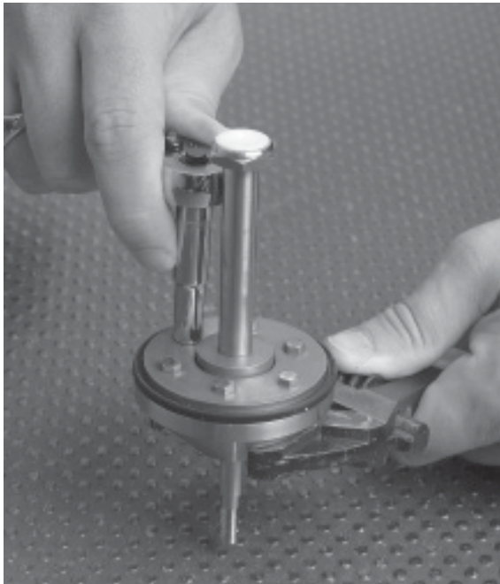
Figure 5. Use Tool Provided or Spring Seat (key 4) and Stem Assembly (key 2) to Align Disc Retainer (key 8)
