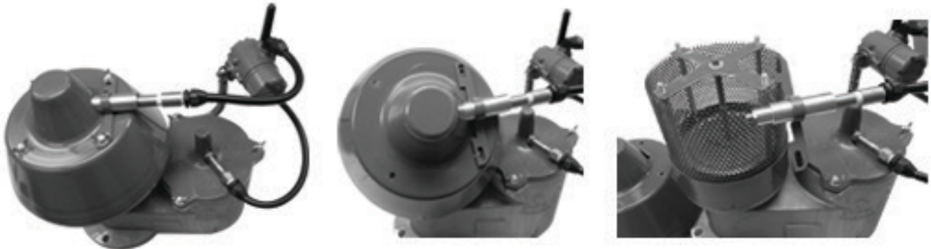
Figure 11. Model ES-950, Installation of Weights
