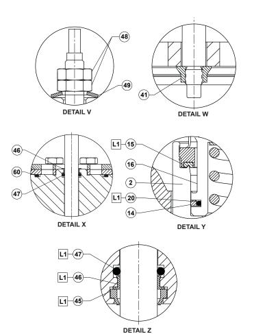
GE38436 APPLY LUBRICANT OR SEALANT<sup>(1)</sup>: L1 = MULTI-PURPOSE PTFE LUBRICANT
