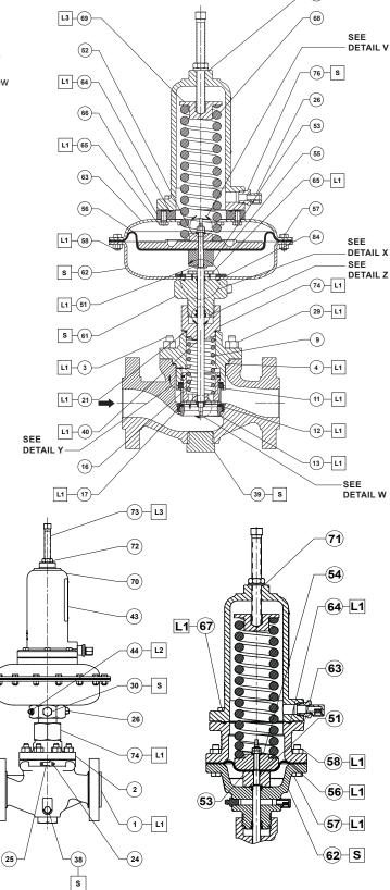
APPLY LUBRICANT OR SEALANT<sup>(1)</sup>: L1 = MULTI-PURPOSE POLYTETRAFLUOROETHYLENE (PTFE) LUBRICANT
