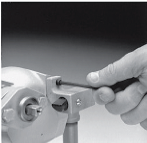
Step 9 Install 3/4 in. / 19.1 mm long bolt through second hole and firmly tighten with 5/32 Allen head wrench.
