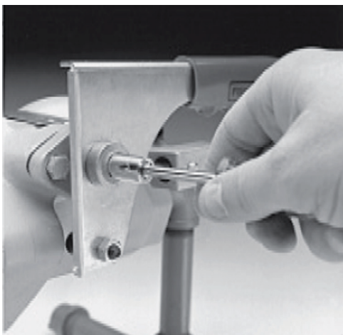
Step 3 Remove handle bolt and handle. Save these two parts.
