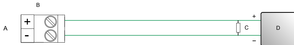
Figure 4-4: Internally-powered FO wiring
