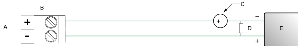
Figure 4-2: Externally-powered mA Output wiring
