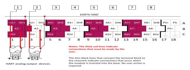
**Note:** All field wiring must be braid-shielded and grounded at the point of entry of the cabinet using the recommended hardware (refer to the *Planning Your Ovation System* manual for information on cabling and grounding).
