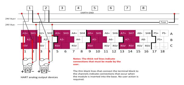
**Note:** All field wiring must be braid-shielded and grounded at the point of entry of the cabinet using the recommended hardware (refer to the <u>Planning Your Ovation System</u> manual for information on cabling and grounding).
