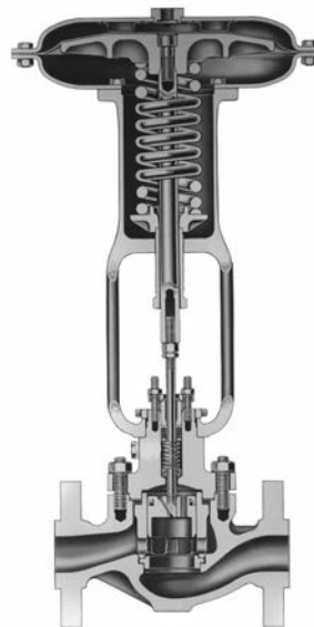
Fisher 655-ED Construction Details
