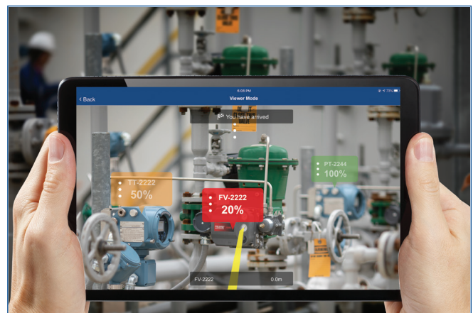
AMS Optics Augmented Reality shows asset data out in the field.
