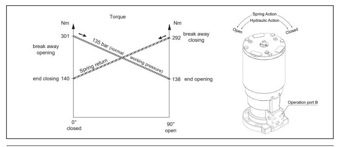
**Note!** The BRCF fail safe actuator is "Fail Close" in the standard version. Optionally a "Fail Open " version can be ordered. In case of Fail Open the above torque curve and operation chart is opposite.
