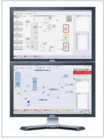
Monitors can also be mounted vertically with the cursor movement set to allow the mouse to move the pointer vertically to access the upper screen.
