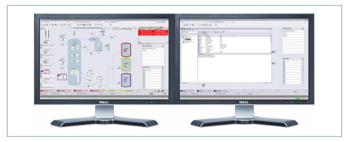
View diagnostics or Control Studio while keeping operating displays in full view. Displays can be exchanged between screens with a single mouse click.
