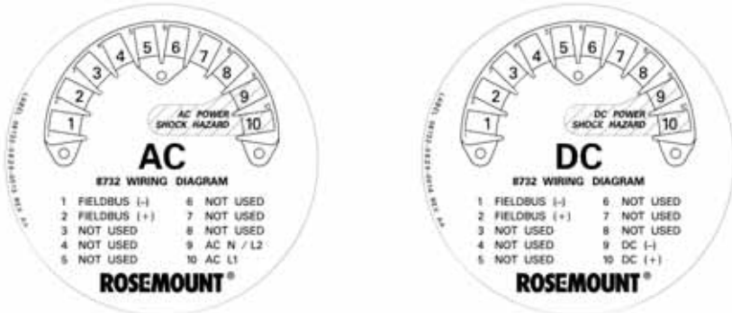
Figure 22. 8732E Transmitter Power Connections
