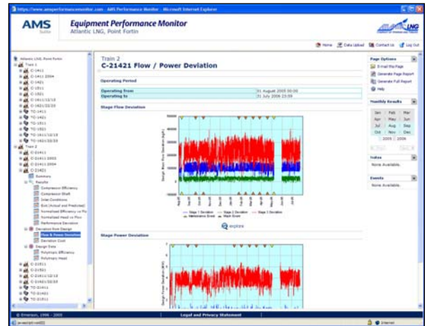
Propane Compressor - Flow/Power Deviation KPI.
