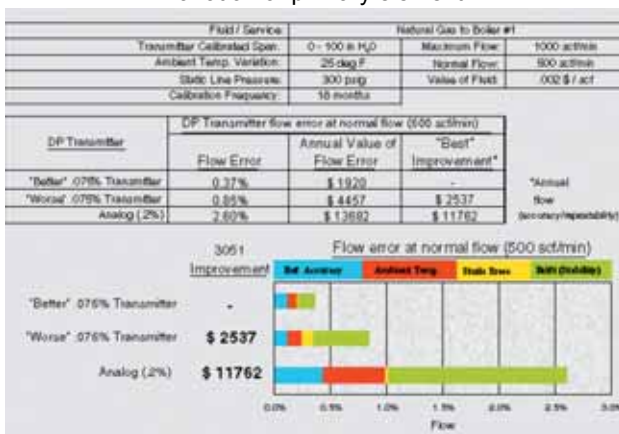
FIGURE 2. Flow Error from DP Transmitter
